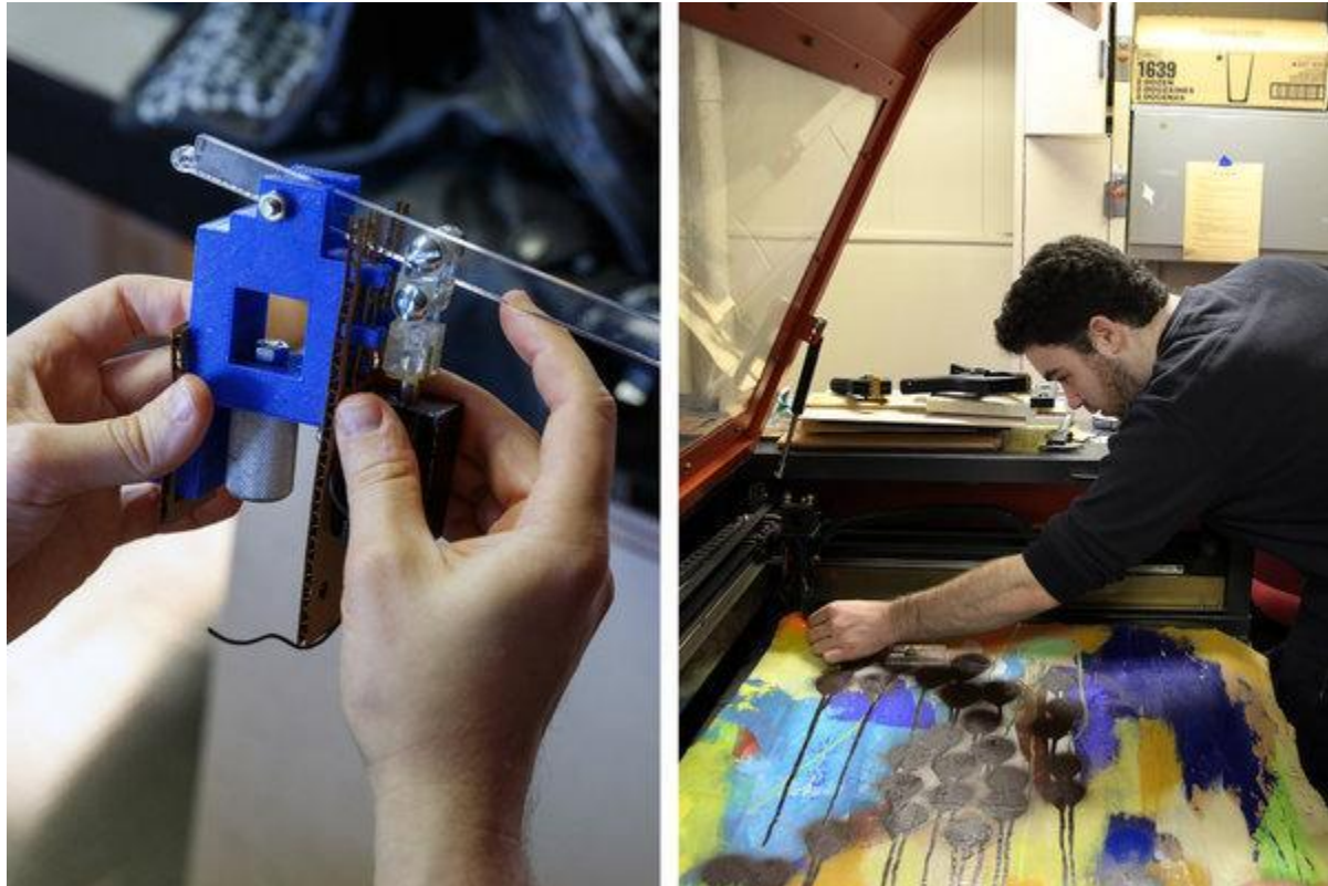
A computer-controlled drumstick was made with a 3-D plastic printer and laser cutter, right (that's a student artwork on the cutter). Credit Richard Perry/The New York Times
