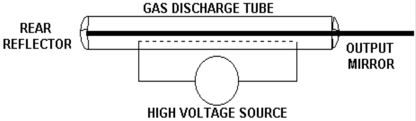
Gas lasers consist of a gas filled tube placed in the laser cavity. A voltage (the external pump source) is applied to the tube to excite the atoms in the gas to a population inversion. The light emitted from this type of laser is normally continuous wave (CW).
